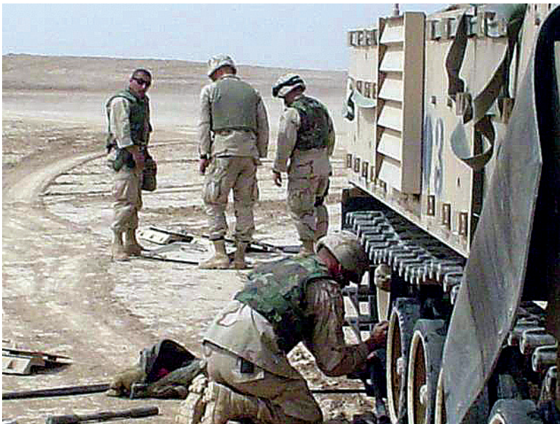
The FIF translator, Koenig, and I (background middle) removed the skirt to give Fogle (foreground) access to the track.
